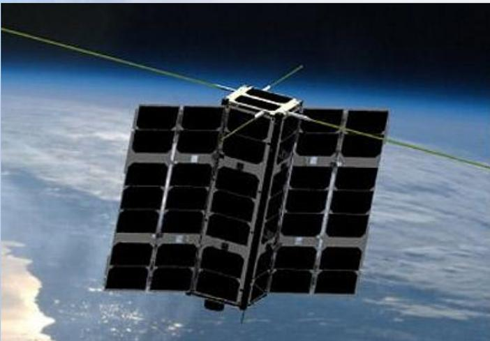
Spire Global satellites provide commercial and government customers with radio occultation data for atmospheric temperature, pressure and humidity that can be vital for forecasting severe weather. Photo credit: Spire Global
