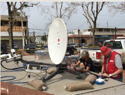
Above) VSAT terminals restoring connectivity in Puerto Rico. (Photo credit: Colin Chaperon for the American Red Cross)
