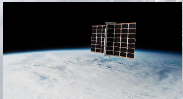
Spire Global satellites like the one pictured above provide commercial and government customers with radio occultation data for atmospheric temperature, pressure and humidity that can be vital for forecasting severe weather. Photo credit: Spire Global
