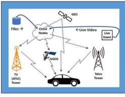
KenCast provides content delivery to fixed-sites and Vehicles-On-The-Move for entities requiring ultra-reliable, ultra-secure operation -- often with e-commerce payment. Our Fazzt platform supports unicast and multicast of files and live video via TCP/UDP, DVB-S2&S2X, ATSC 3.0, 5G, eMBMS, and fiber optic CDNs at speeds up to 600 Mbps."
